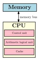
CPU and main memory is connected via the memory bus.
