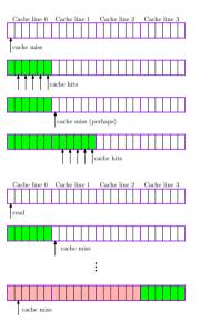
Latency – how long the CPU has to wait between issuing a memory request and receiving the first byte – is an important performance consideration.
